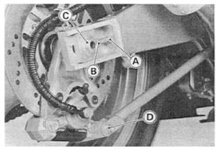
A. Locknut B. Adjuster C. Axle D. Torque Link Nut
